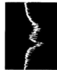
Fig. 14. 455 kHz felle (trap). Signal: U_n = 200 mV via wobblor/S.K.A. (fig. 15/16) tilført (applied) M14. Oscilloscope: Vert.: 50mV/div. Hor.: 2 kHz/div.
