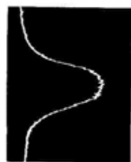
Fig. 13. MB-MW Signal: U_n = 100 V via wobblor/S.K.A. (fig. 15/16) tilført (applied) M14. Oscilloscope: Vert.: 200 mV/div. Hor.: 2kHz/div.
