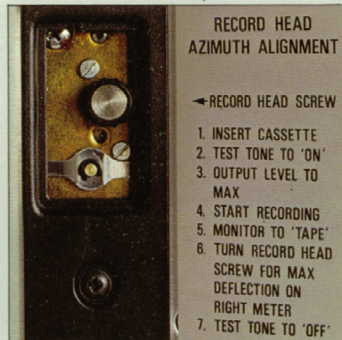
The record head azimuth adjustment.
