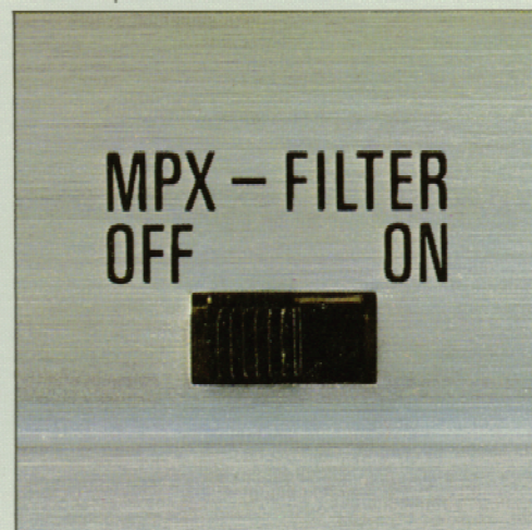
The multiplex filter can be switched in and out.
