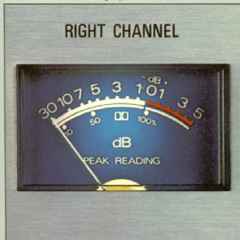
The TCD 330 has large peak meters.
