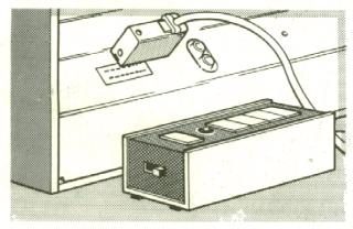
Connect the Remote Control Unit L'ur to the REMOTE CONTROL socket on the connector strip at the rear side of the tope deck.
