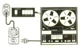
NOTE! When the tape deck are not going to be started or stopped with the automatic timer, the slide switch TIMED START on the Remote Control Unit shall always be in the position OFF.
