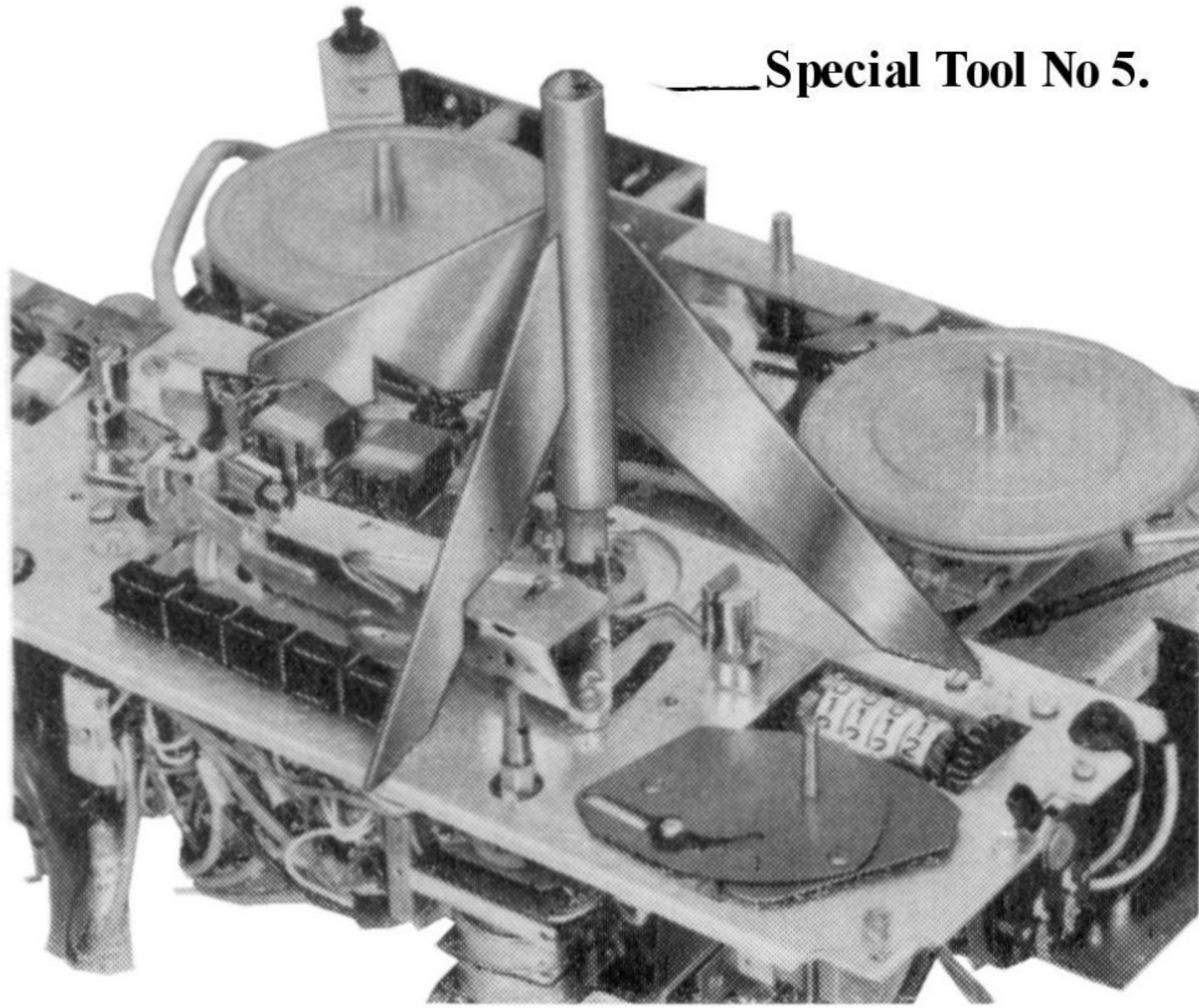
Fig. 32. Alignment of the capstan with tool No. 5.
