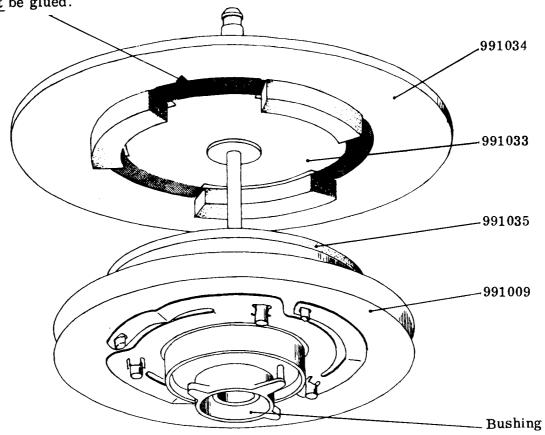
Bottom view of take-up turntable and friction disc.
