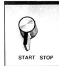
By means of the START/STOP switch the tape can be instantaneously stopped during recording or playback.
