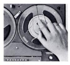
Pull out sufficient tape to form a loop on the right hand side. Insert the tape in the slot in the reel and hold the tape end in position while turning the reel anti-clockwise until the tape is taut.
