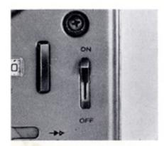
Pull out the mains lead from the recess at the rear of the tape recorder. Plug into a mains socket and switch on.
