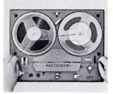
Cut off the length of self-adhesive tape on the end of new tapes to avoid the risk of depositing adhesive on the heads. Place a full reel on the left hand turntable. Hold the tape taut between forefingers and thumbs and insert it in the tape slot, ensuring that the shiny side is towards the front of the machine.
