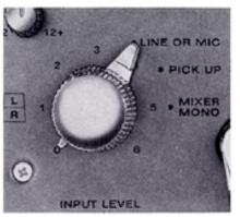
Set the input selector to LINE OR MIC thereby connecting the line/microphone sockets to their respective input amplifiers. In mono recording (only one function selector in REC) the outputs of the input amplifiers are connected together and the programme can therefore be fed to any one the MIC inputs. The signal level is set by means of INPUT LEVEL for the input in use.
