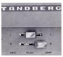
With the function selector for channel L in the PLAY position, move the function selector for channel R to the AMP position. When playing back from channel R, set the function selector for channel R to PLAY and channel L to AMP.
