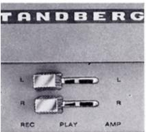
Set both function selectors to REC and hold in position while moving the tape motion lever to the  $\rightarrow$  position. The function selectors are now locked in the REC position, and both recording indicators will light up.
