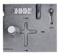
Rewind the tape to the position where recording started, by moving the tape motion lever to the <- position. Stop rewinding by moving the tape motion lever to the neutral position when the correct position is shown on the tape counter.
