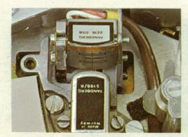
tape passes between the two heads. The Cross-field head allows the tape to accept much stronger signals than is possible with conventional recording techniques, thereby improve the dynamic range and extending the frequency response.
